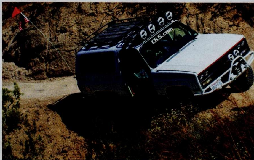
▲ Here's a good candidate for a two-way pull. It needs to be pulled forward and left at the same time.
