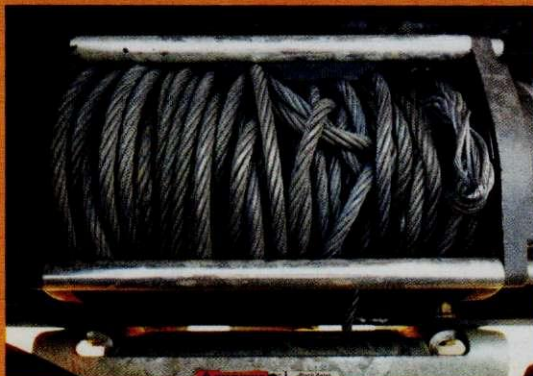
▲ A destroyed winch cable
